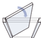
Clockwise closing Left hand ISO. 5.0
